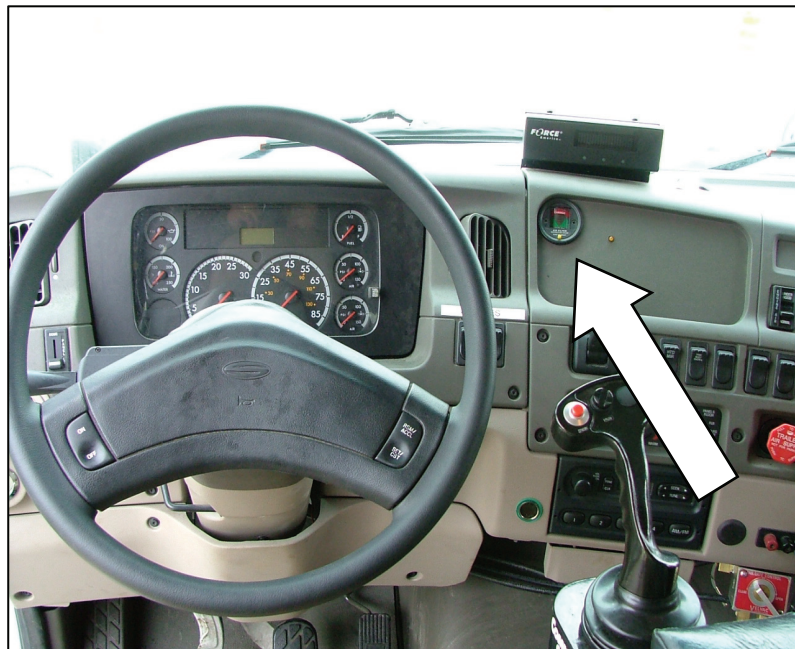
Figure 4-22 Air filter indicator located inside the truck cab
