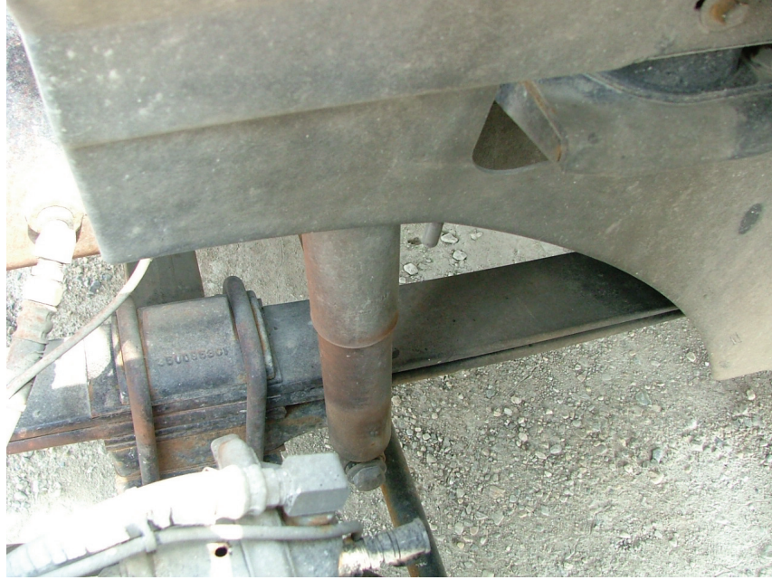
Figure 4-13 Truck shock absorber
