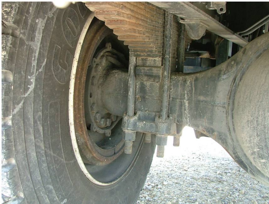
Figure 4-27 Truck rear axle spring leaves
