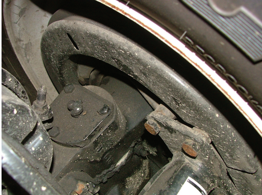
Figure 4-10 Dump truck front brake drum
