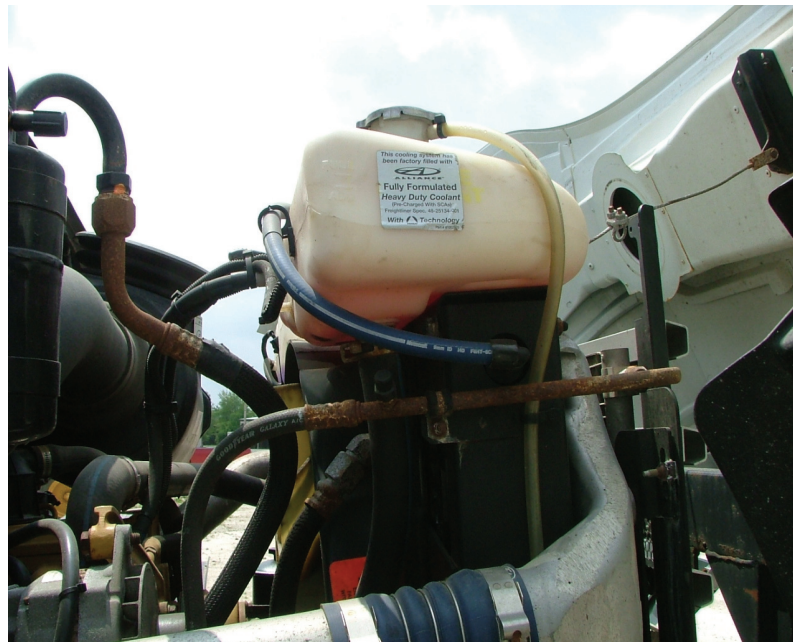
Figure 4-4 Dump truck coolant level fill bottle
