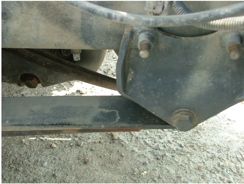
Figure 4-11 Spring mount at truck frame
