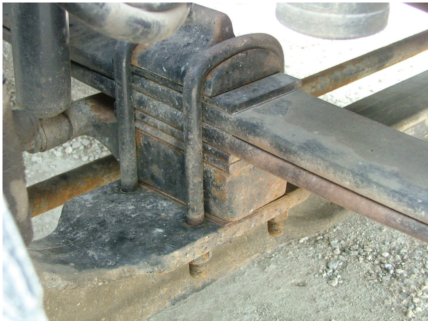
Figure 4-12 Truck spring shackle
