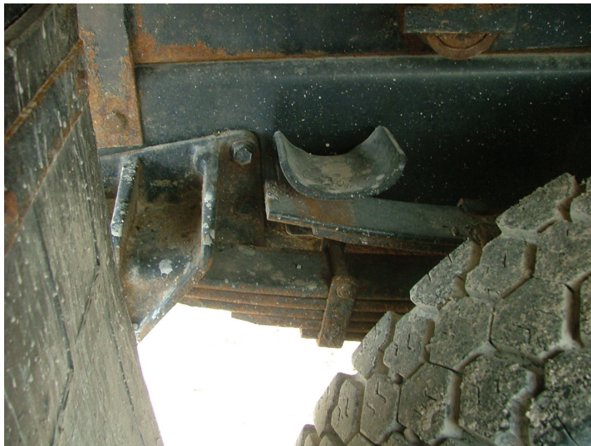
Figure 4-29 Truck rear spring mounts
