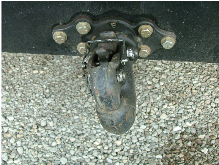
Figure 4-31 Truck mounted pintle hitch
