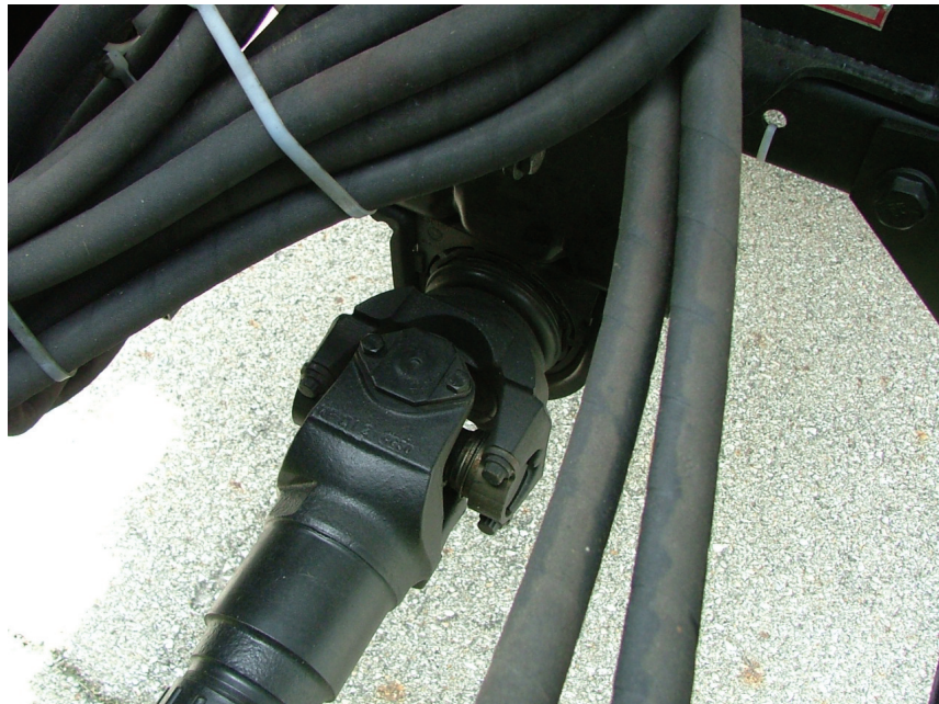
Figure 4-33 Drive shaft universal joints
