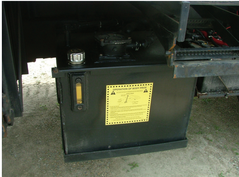
Figure 4-21 Hydraulic fluid tank with sight glass
