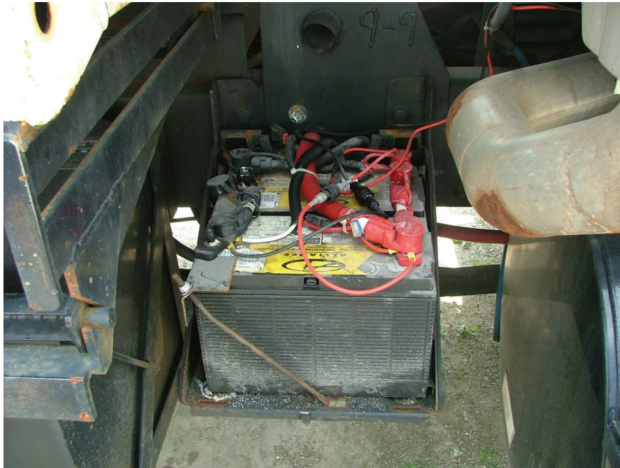
Figure 4-35 Truck battery box and batteries
