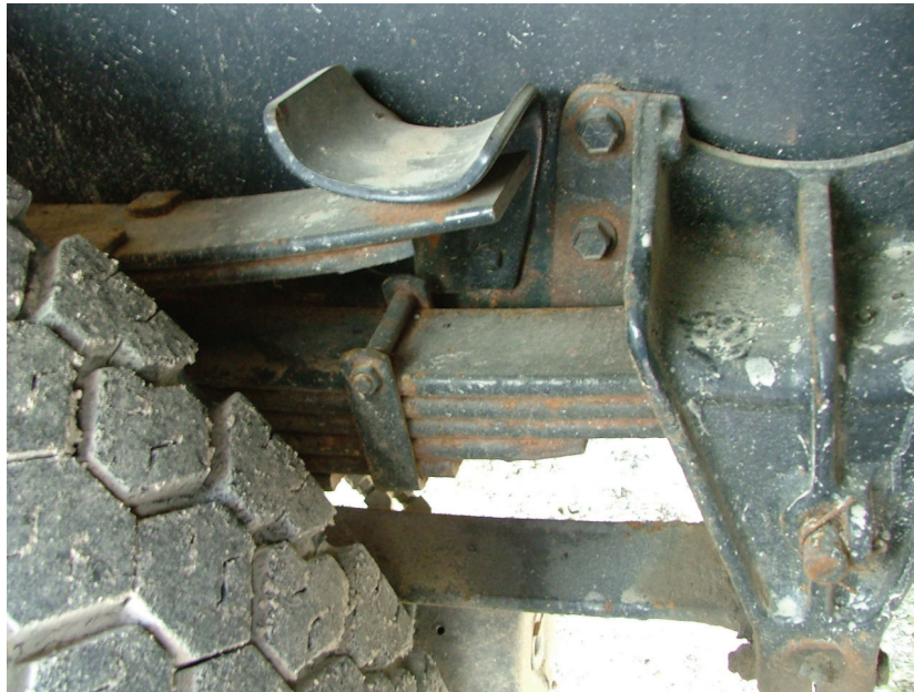
Figure 4-28 Truck rear spring mounts
