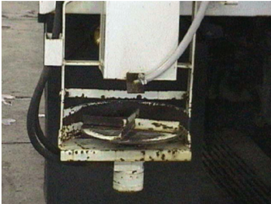
Figure 12-14 Tailgate spinner showing pre-wetting material with brine
