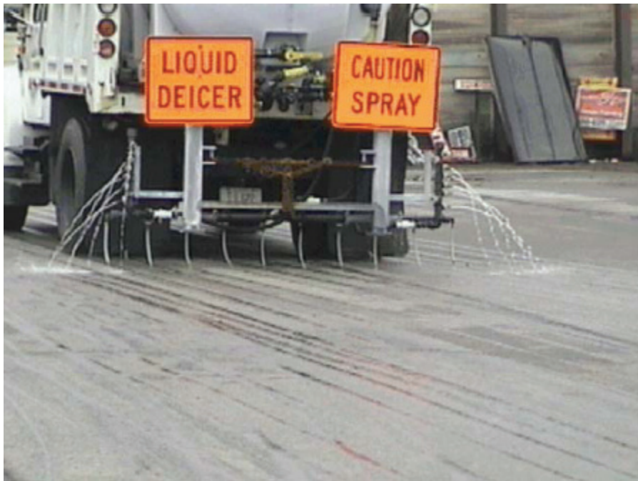
Figure 12-11 Brine tank insert with bottom and side spray bars
