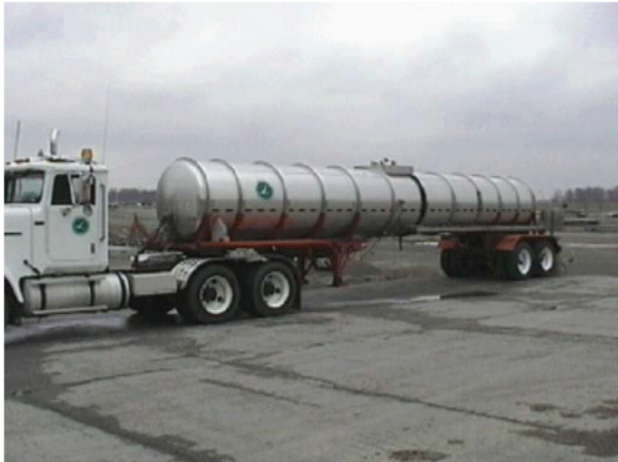
Figure 12-9 Side view of brine semi tank
