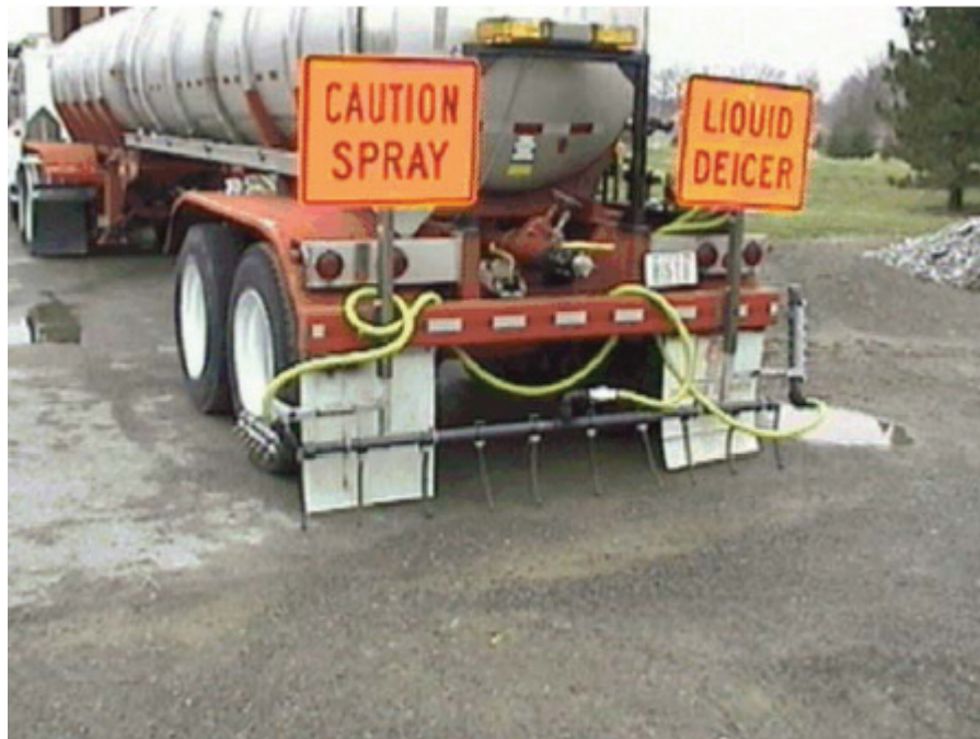
Figure 12-10 Rear view of brine semi tank
