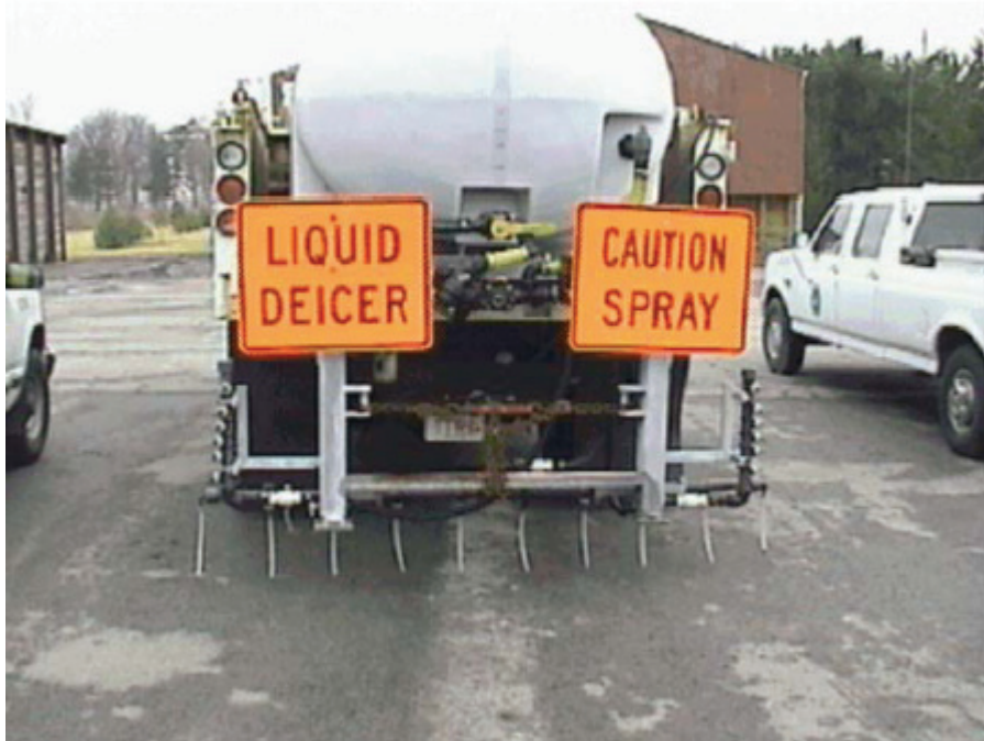
Figure 12-8 Brine insert tank with spray bar
