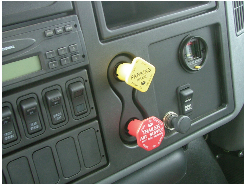
Figure 6-1 Truck and trailer parking and emergency brake controls
