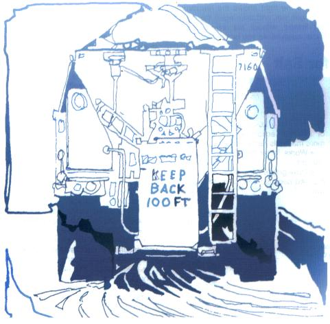
Prewetting brine can be added to the load at the yard, (see next page) or during spreading operations using saddle tanks, shown here, or home built "over-cab" tanks.
