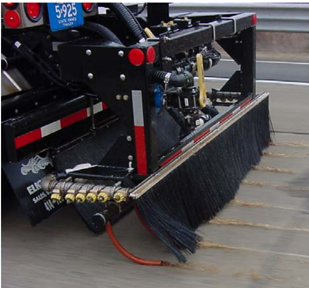
Figure 2: Anti-ice rig equipped with rubber application hoses
