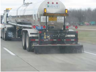
Figure 1: A semi-trailer equipped for anti-icing
