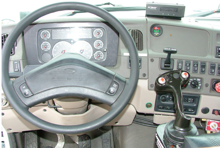
Figure 3-3 Sterling Cab with Force America hydraulic control
