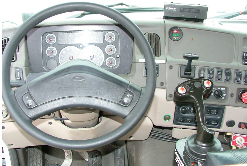
Figure 3-3 Sterling Cab with Force America hydraulic control
