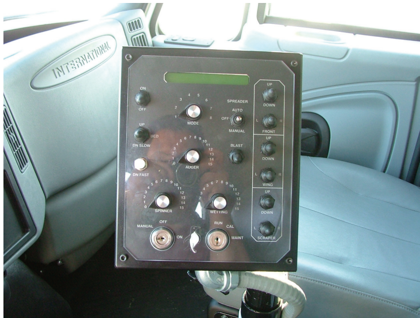
Figure 3-4 Pengwyn hydraulic control
