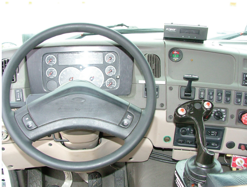
Figure 3-3 Sterling Cab with Force America hydraulic control
