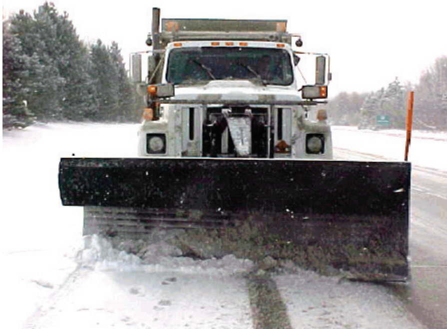
Figure 12-16 Dump truck with a front plow
