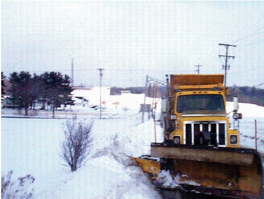
Figure 12-17 Dump truck with a front plow and a wing plow
