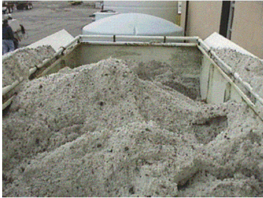
Figure 12-1 Salt brine mixing hopper
