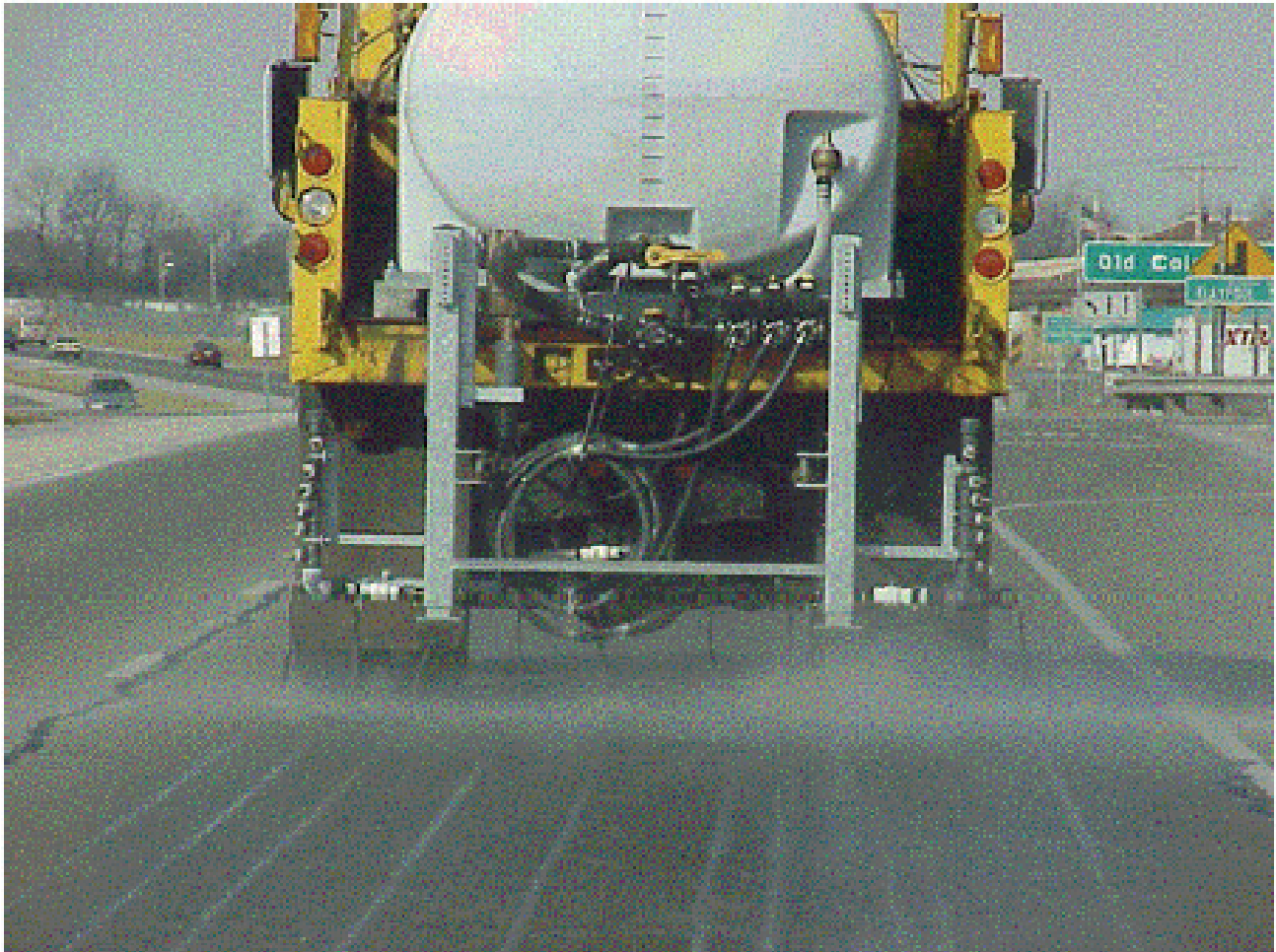
Figure 12-3 Brine applicator, applying pre-treat
