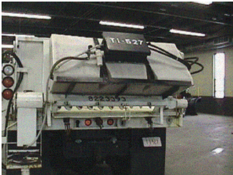
Figure 12-6 Tailgate mounted brine tank
