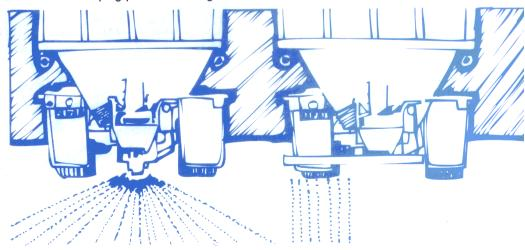
Spreading can be done full-width or windrow. Both have strengths depending on conditions. Pay special attention to spinner speeds. A spinner that revolves too fast will throw salt over a wide area, possibly wasting material. You may correct "overthrow" by adjusting the drop location on the spinner by using your directional baffles or reducing spinner speed. Traffic density and highway design largely determine the spreading pattern required.
