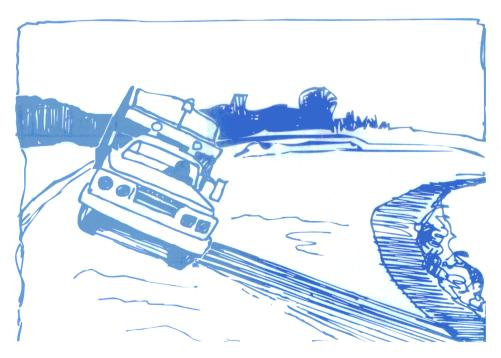
Salt bridges first. Bridges freeze long before road surfaces because they do not hold warmth as a roadbed does, since cold air reaches both the top and bottom surfaces of bridge decks. They should receive early attention and an application of salt. Bridge decks may ice over even when there is no precipitation because of high humidity and low temperatures. (Or under certain other conditions, bridges will frost over without precipitation and must be salted.)
