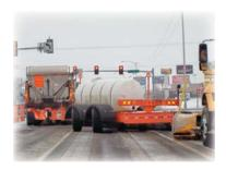
Operators have found that in large multilane intersections retracting the Tow Plow enough to clear traffic and obstacles allows for a large area of the intersection to be cleared in one pass. Good judgment and communication with operators of single front plow trucks may be necessary to provide efficient clearing of large multilane intersections.
