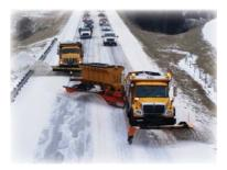
results while reducing snow removal costs for equipment, fuel and labor. The Tow Plow is a large piece of equipment and requires a skilled operator. Proper training, knowledge and experience are essential for an operator to maximize the Tow Plow's benefits in snow removal operations.
