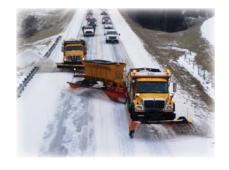
operator decides to close in on obstacles, such as guardrails or curbs, be aware that the snow load could suddenly reduce and the Tow Plow will skew back to its original position and may strike roadside obstacles. This situation is even more prevalent when plowing under overpasses and bridges as the snow load decreases under these structures.
