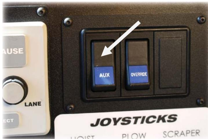
If used in conjunction with the ACS spreader controls, the operator can deliver an additional 15 gpm from the ACS system giving a total output up to approximately 30 gpm hydraulic oil flow depend on the Rate setting of the ACS.
