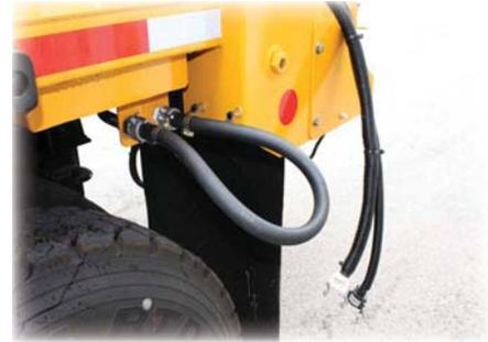
Install a jumper hose to both cam lock couplers to create a loop from the suction to the pressure side of the liquid system on the truck.
