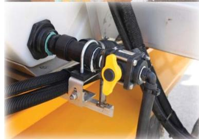
Once fresh water is supplied to the nurse tank/system, operate liquid pump in manual mode for several minutes discharging water from black cam-lock coupler to flush contaminants from system.
