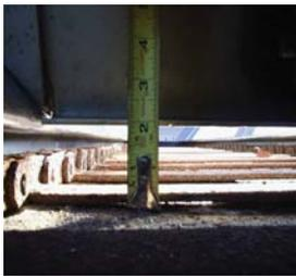
The gate should also be checked at this time for proper operation. Gate heights are crucial for calibrating and the operation of the truck. When measuring gate heights, measure from the body floor and not the bed chain. Improper gate heights waste salt and lead to misjudged stockpile figures. The gate should be checked before each storm and after each material change
