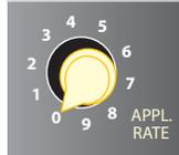
The Application Rate knob is used to increase or decrease the actual application rate that is being applied. The rate at which this happens depends on the material that is selected. Example Salt @ 100, 150, 200lbs/mi., with 0 being 0, 1 being 100lbs/mi, 2 being 150lbs/mi and so on up the scale.
