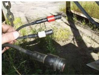
Once this is complete move to the outside of the cab. With a front dump check the connections at the conveyor sensor to see if it's broken or the wire has been chaffed or cut. Also check for major hydraulic leaks that could lead to a problem.
