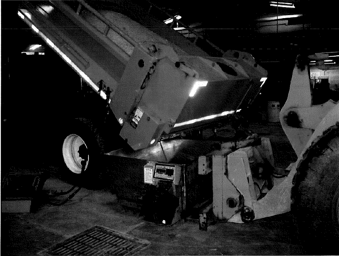
Figure 3 - Raising the Dump Body
