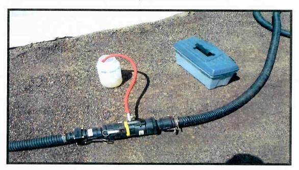
After the tanker has emptied approximately 1/3 of the Magnesium Chloride Product into the CDOT storage tanks, the pumping is to be stopped and the same delivery hose is to be used to fill 1/2 of the sample container.
